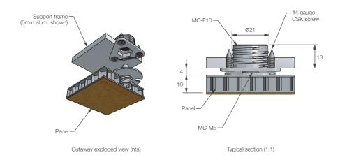
The Fastmount<sup>®</sup> multi-award winning system has revolutionized the mounting of panels. Panels can easily be removed and refitted in any sequence time after time. For further information or technical support contact: info@fastmount.com
